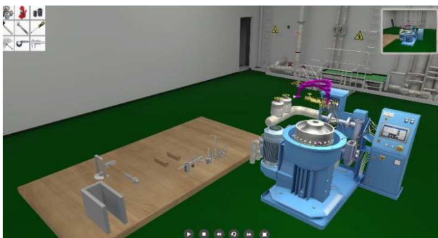
Figure 10. Virtual disassembly rendering of marine oil separator.
